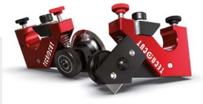
*The CSU - Compact Slitting Unit is a stand-alone slitting unit that stands out due to its simple assembly and adaptability. It can be equipped with either rotary or razor blades, allowing to make precise longitudinal cuts or longitudinal perforations. Thanks to its exchangeable design, the blades can be adjusted to perform full cut (die cut) or half cut (kiss cut), depending on the customer's specific needs.*
